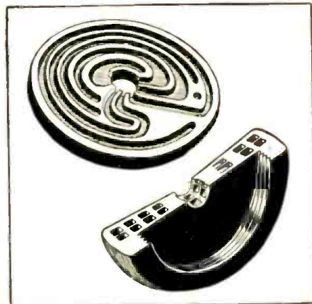
Cut-away views of the new high-quality earphone cap. No. 632
