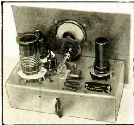
Rear view of set, showing plug-in coil and two tubes in place.
